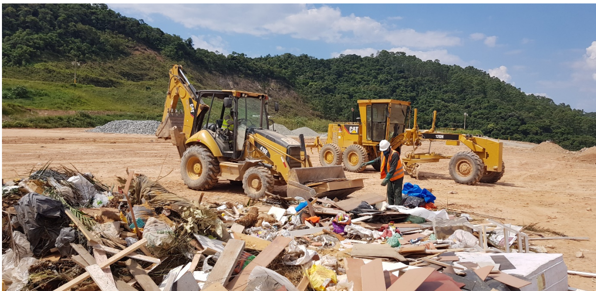
Figure 15 Photo of an operator loading the backhoe's shovel in the sorting area
